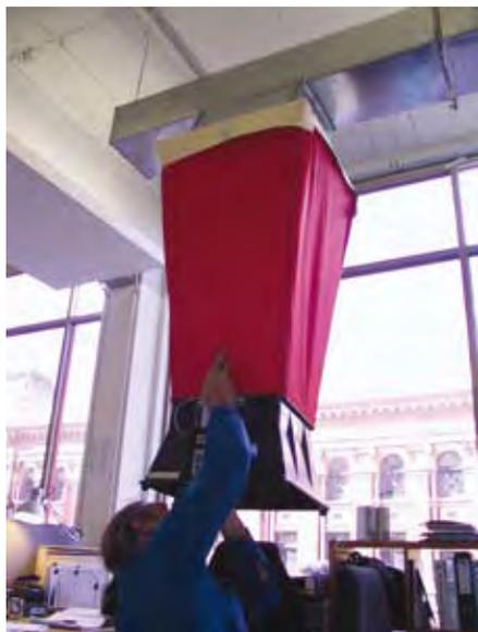
Checking air flow readings from supply air diffuser
