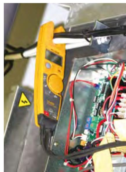
Typical clamp meter used by HVAC technician to check correct electrical current
